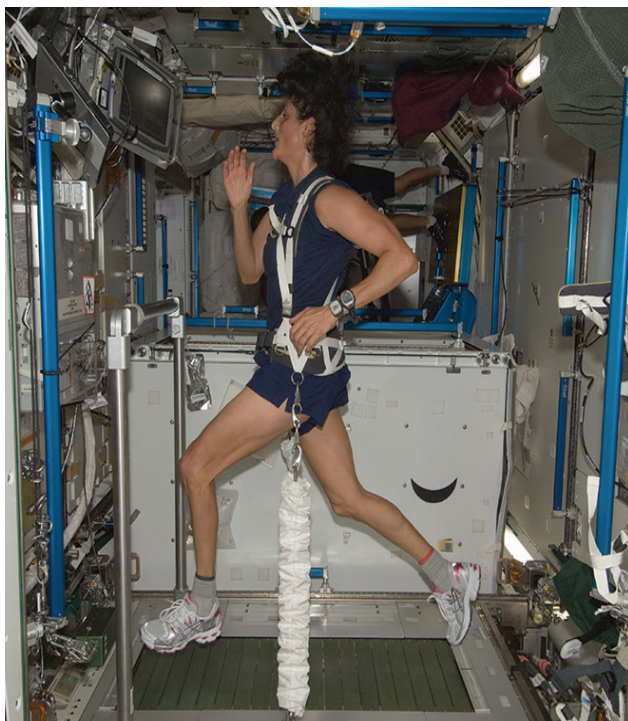
Figure 24-7. NASA astronaut Sunita Williams, Expedition 32 flight engineer, equipped with a bungee harness, exercises on the Combined Operational Load Bearing External Resistance Treadmill (COLBERT) in the Tranquility node of the International Space Station, 2012. NASA photo ID: ISS032E011701. Reproduced from: https://images.nasa.gov/details-iss032e011700.html .
